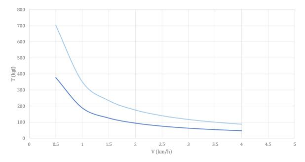
Figure 5.1. Maximum generated traction force (T) versus speed (V) for one (dark blue) or two (light blue) draught animal(s).
