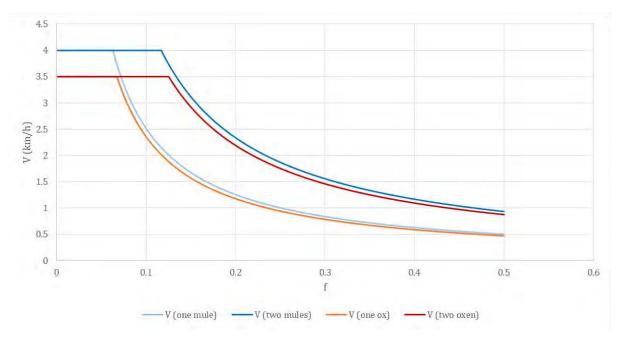
Figure 5.2. Speed (V) versus the friction coefficient (f) for mule- and ox-carts drawn by one or two animals.
