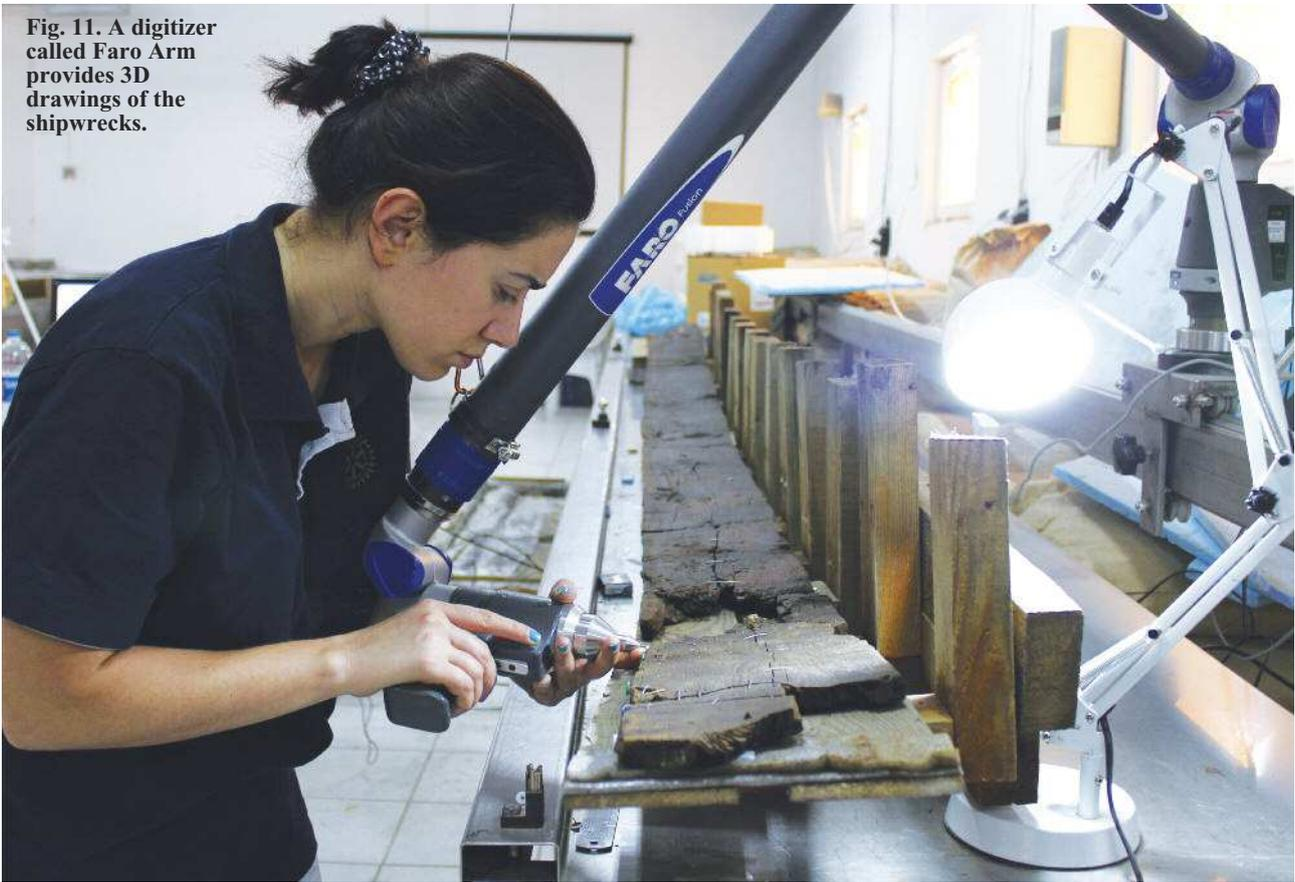
Detailed recording of the surviving ship timbers are made with a 3-D digitizer called, *FaroArm* are made. This technology has been used in the field of archaeology for the first time in Turkey by Istanbul University's Project team (**Fig. 11**). Ascertainable details of each timber, such as fastenings, joints, angles, tool marks, corrosion stains, etc. are all recorded using the laser scanner. Each digitized timber can then be used to create 3-D images of ship timbers<sup>10</sup>.
