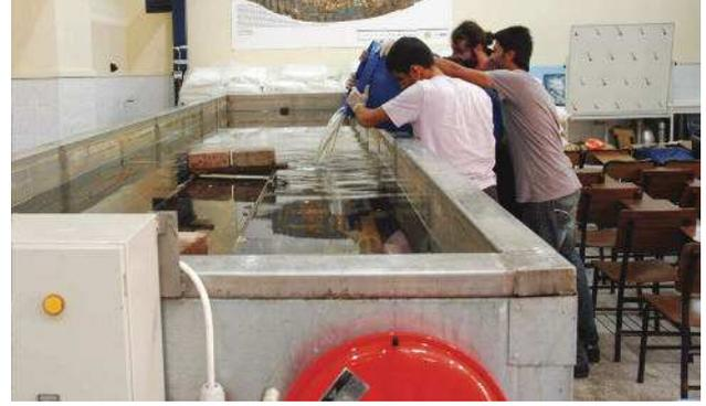
Fig. 17. PEG solution is being poured into the conservation tank.
