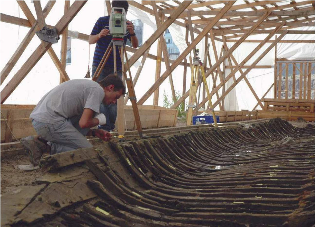
Fig. 6. A detail from Total Station work that provides 3D field drawings.
