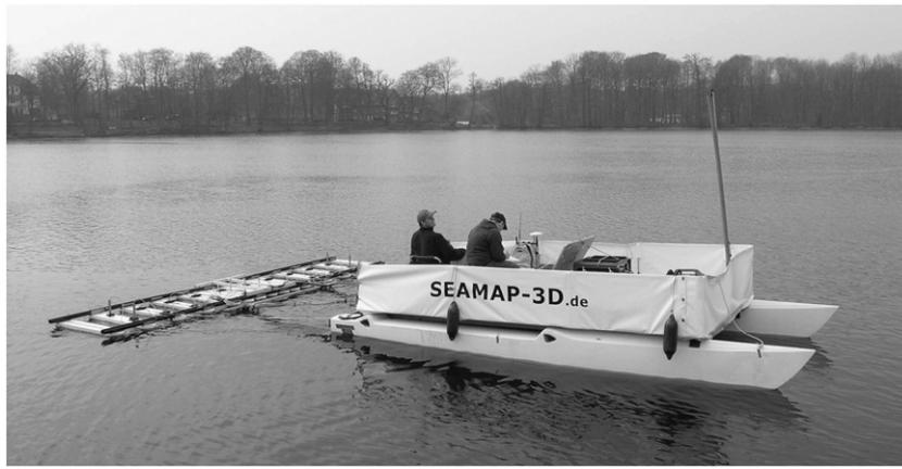
**Fig. 1.** SEAMAP-3D ultra-high-resolution seismic acquisition prototype on a lake in Northern Germany. A refitted catamaran is used as the acquisition vessel. It is towing the boomer seismic source and the rigid frame hydrophone array.
