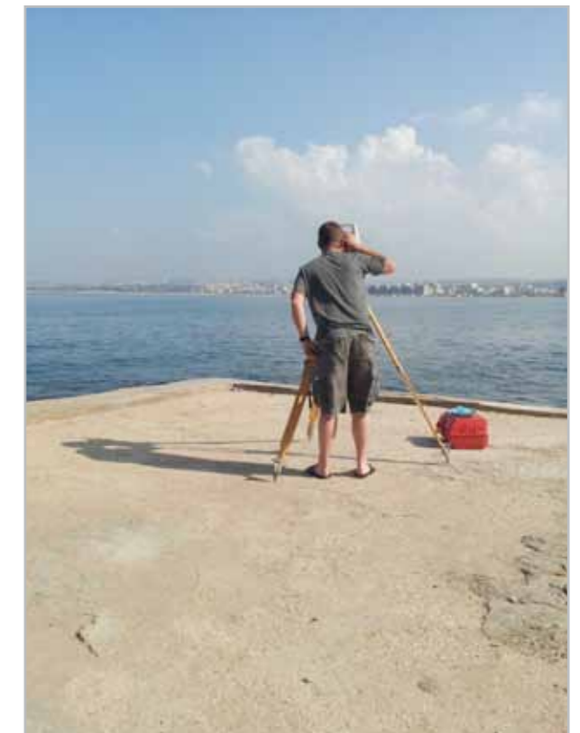
Fig. 6- Archaeologist using Leica 1200+ Total Station for topographic survey at Northern Harbour of Tyre, looking east.
