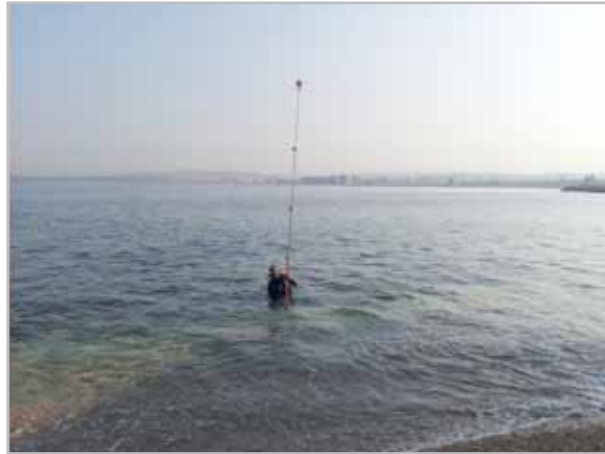
Fig. 7- Archaeologist using Stadia Rod for Underwater Survey at Northern Harbour of Tyre, looking east.
