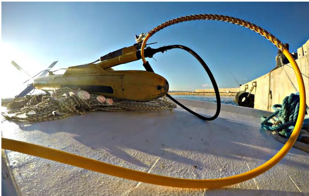
*Fig.3.3.1. The EG&G 272 TD side scan sonar*
