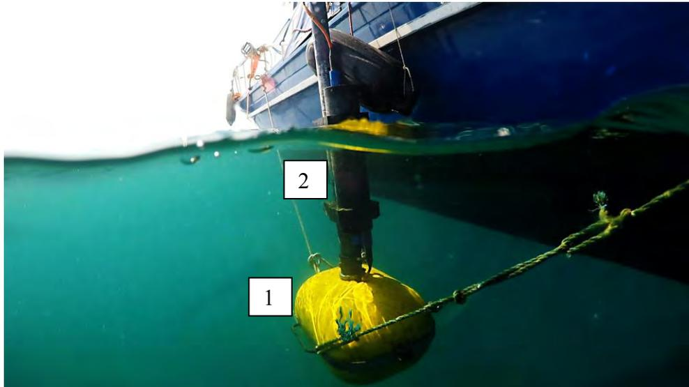
*Fig.3.1.1. O.R.E. Model 138C over-the-side Transducer Mounting (1) and waterproof digital profiler electronics bottle (2).*
