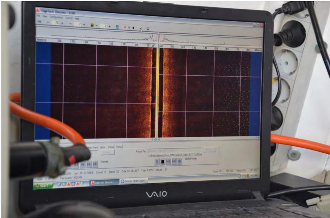
*Fig.3.3.2. The Side Scan Sonar digital recording unit.*
