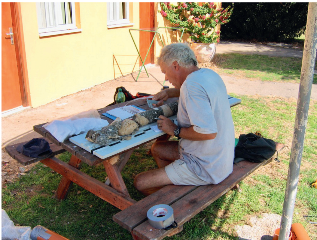
Figure 2.5: A preliminary field analysis of a marine concrete core sample by J.P. Oleson. Large pieces of aggregate and lime are visible (ROMACONS Archive).
