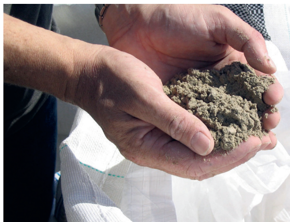
Figure 2.2: Pulvis Puteolanus from the Naples region (ROMACONS Archive, after Brandon et al. 2014: Fig. 1.1).
