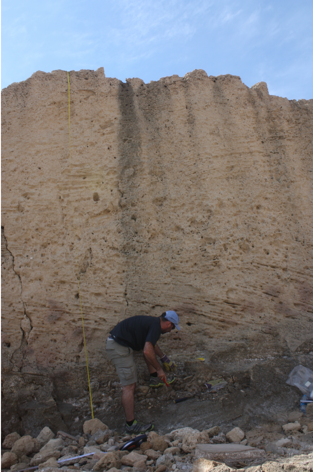
Fig. 2: Rock sampling of the quarry floor for cosmonuclide dating.
