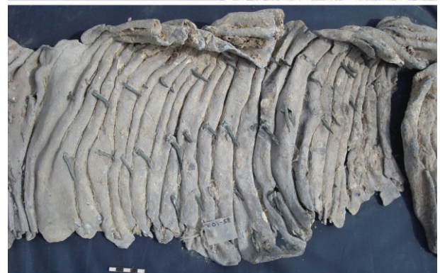
Figure 4. A lead section from a Roman ship's keel, lost after scraping the Akko reef. (E. Galili)
