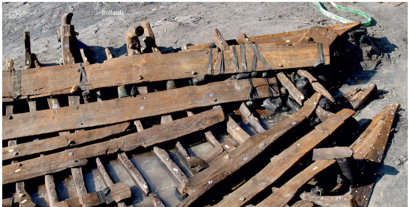
Figure 5.13. The port side of Isola Sacra 1 preserved up to the gunwale showing the two bollards and, on the right, the transom lying under the upper stringer. (Photograph: G. Luglio.)
