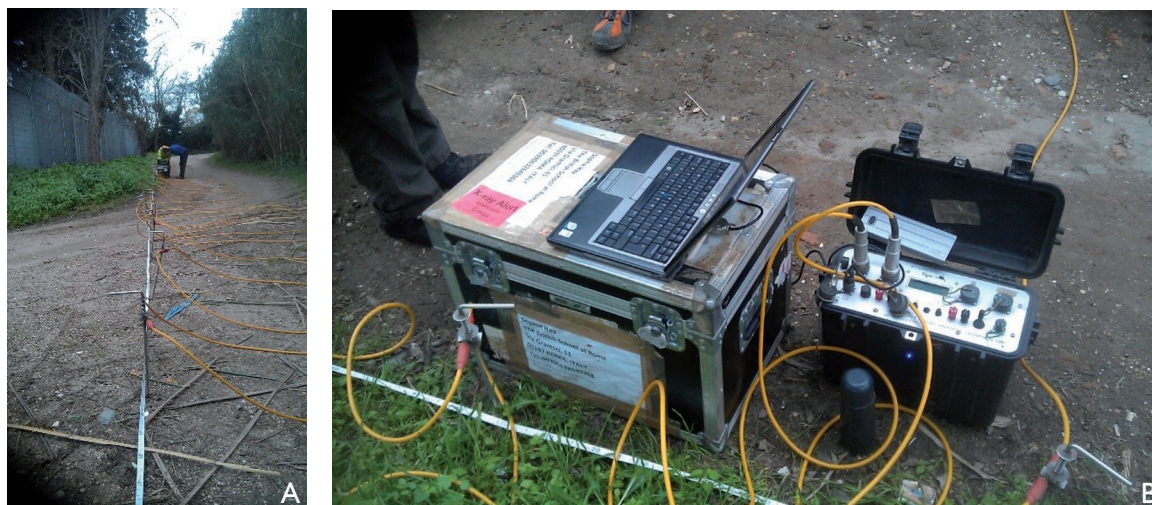
Fig. 3 : (A) Setting out of the ERT probes and checking on the Tigre ; (B) The Allied Associates Tigre Resistivity meter during the ERT survey (K. Strutt).
