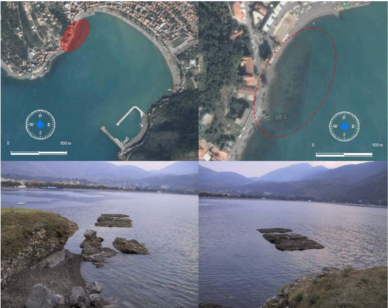
Figura 18 - Satellite views and photographs of the semisubmerged remains of a Roman caisson breakwater in the gulf of Sapri
