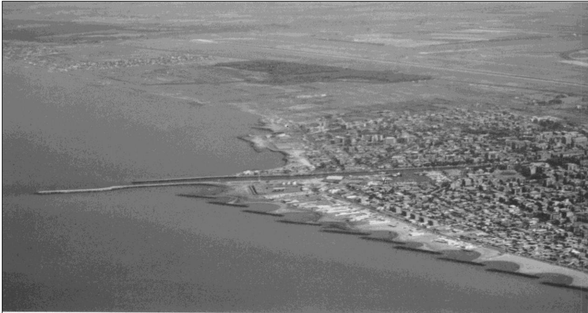
Figure 13.5: The use of offshore breakwaters at the updrift side of a port entrance, Fiumicino (Italy)
