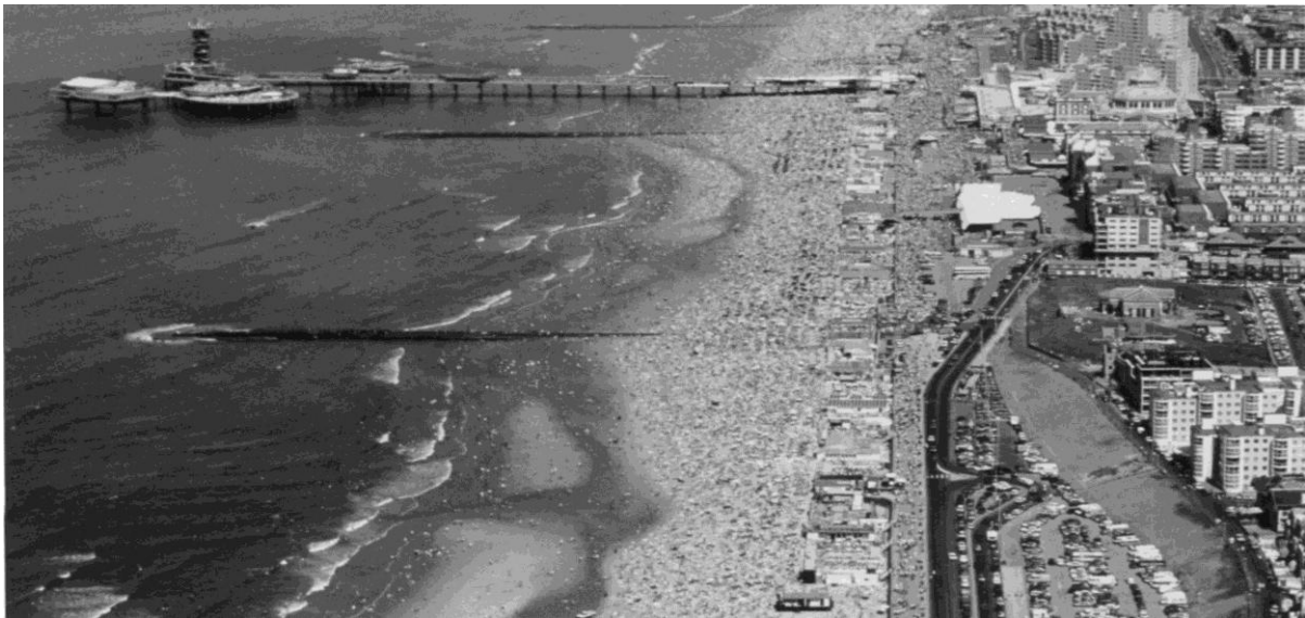
Figure 10.2: Application of groynes at Scheveningen, The Netherlands
