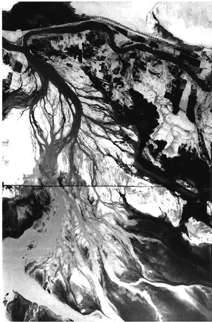
Figure 5A: The Kut barrage on the Tigris between Sheikh Sa'ad and Ali al Carbi drains excess flood discharge into Lake as Sa'adiya. The barrage maintains and augments a natural flood splay. Source: KH4B_1103-1A-D041-056 (May 1968). 2X enlargement to scale ~1:75,000.
