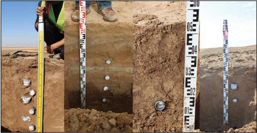
Figure 8. Samples being taken for OSL dating. Left to right: site 1, site 3, site 5 and site 4 (figure by authors).
