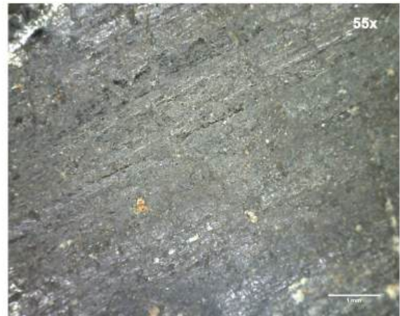
BRW Sample SUM10C; US174, 78 with sand, mica plant/vegetal temper and organic yellow inclusions . Surface slipped and burnished
