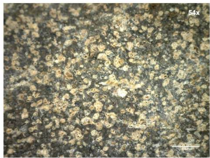
Khor Rori Black and grey ware sample (SUM10C US425, 7) (54x) - surface pitted with lime and organic impurities
