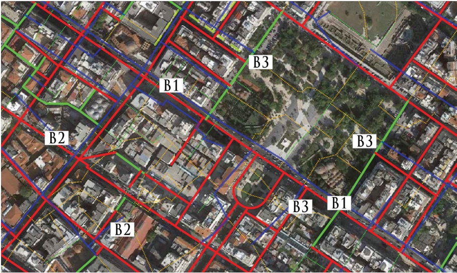
Fig. 4: The typology used in the street network analysis. Examples of rectified streets, according to the typology in the text, pointed on a fragment of the plan illustrated in Fig. 3-left. Base: Google Satellite imagery. B1 = streets with an offset axis; B2 = streets with a (slight) change of direction; B3 = relocated streets. The line codes are as follows: green = old street, preserved; blue = old street, rectified (the old axis); red: new street (newly cut; or rectified, the new axis); dotted green = streets which disappeared but might have left traces in the urban print (alleys, limits of properties, or of buildings); dotted yellow = streets which disappeared without apparent trace in the present footprint.
