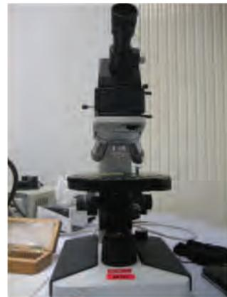
**Microscope polarisant Leica**
