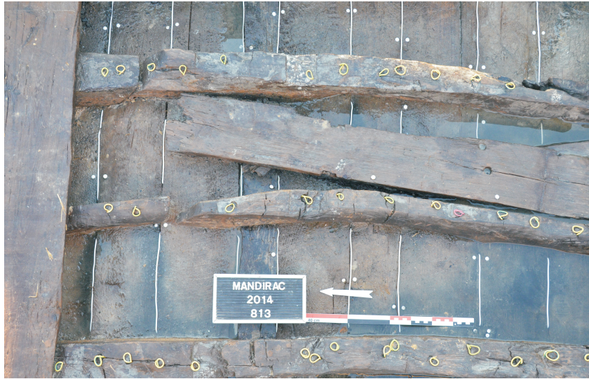
Fig. 12: Notches on either side of the keel on each of the frames 6, 7, 8 and 9.
