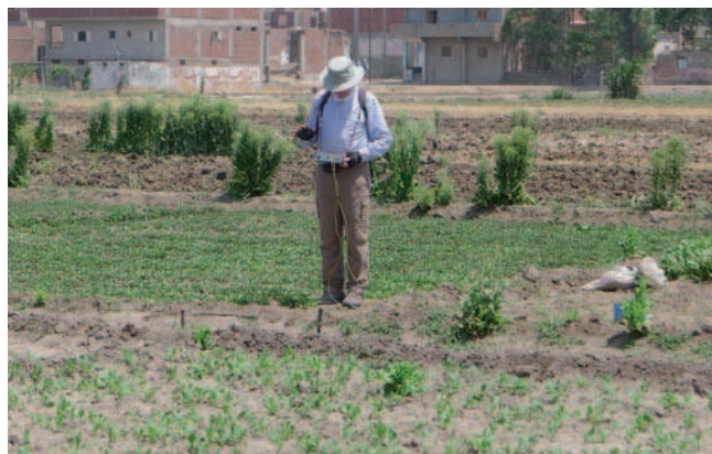
Tomasz Herbich carrying out the vertical electrical sounding survey
