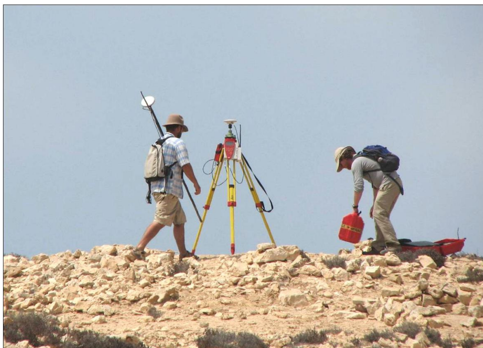
Fig. 7. Julian Whitewright and John Cooper setting up the RTK system for the topographic survey on site 208 at the northern shore of the lake.
