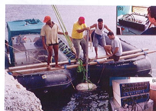
Figure 5: 3.5 kHz sub-bottom profiler: (a) an over the side 4-array transducer, (b) E.P.C. Graphic Recorder, (c) GeoPulse Transmitter and Receiver
