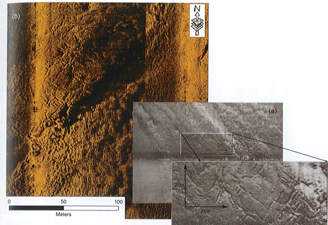
Figure 20: Side scan sonar images (a, b) showing the surface of the Ridge -I. It presents a backscatter geometrical pattern made of patches or smaller strips of high reflectivity
