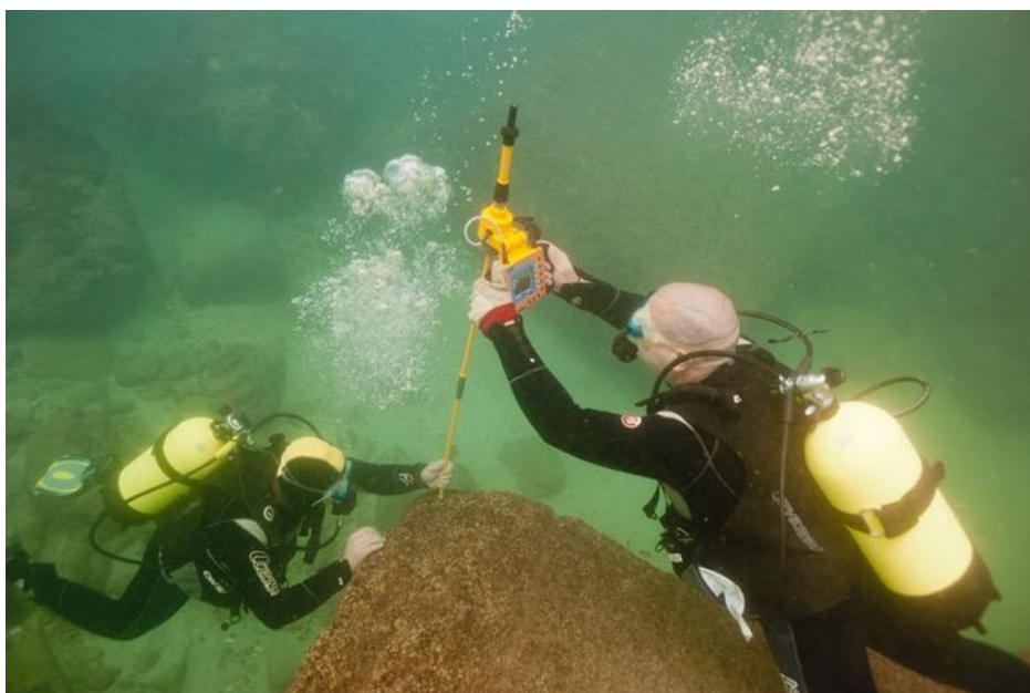
Figure 5. Collecting survey points using the pointer of the Aquameter D100 system (CEALex Archives).
