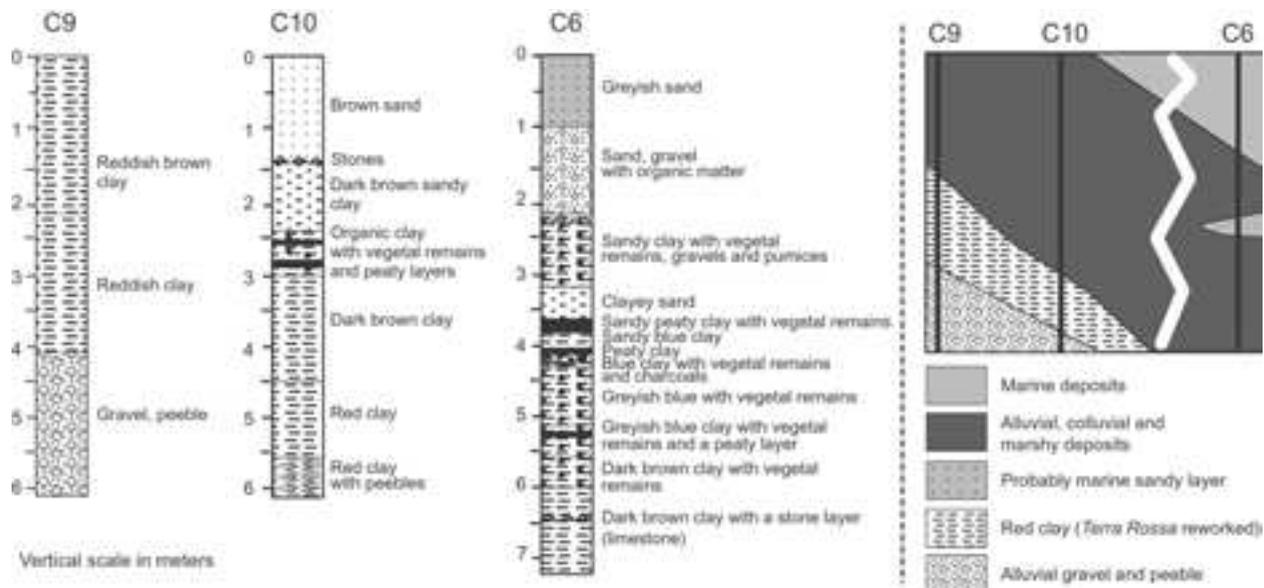
Fig. 2c. Cores in the marsh on its borders (from west to east) and schematic transect.
