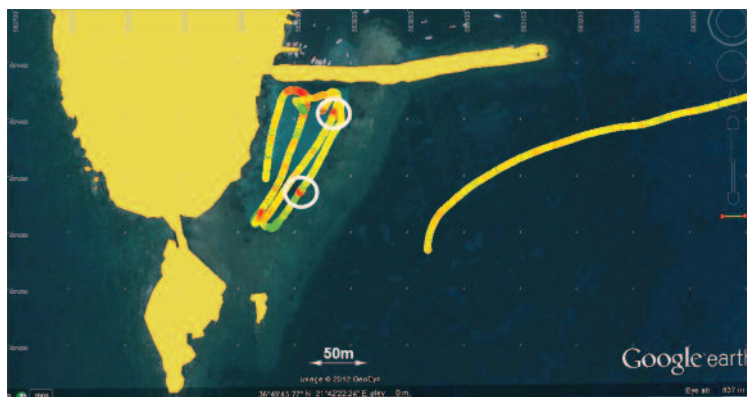
Fig. 6: Visualisation of the magnetic profile of a harbour through a Geographic Information System. Potential artefacts are indicated by the red dots (in the white circles) overlaid on geospatial (coastline) data and Google Earth imagery. Datasets: The GE.N.ESIS Project and courtesy HNHS.
