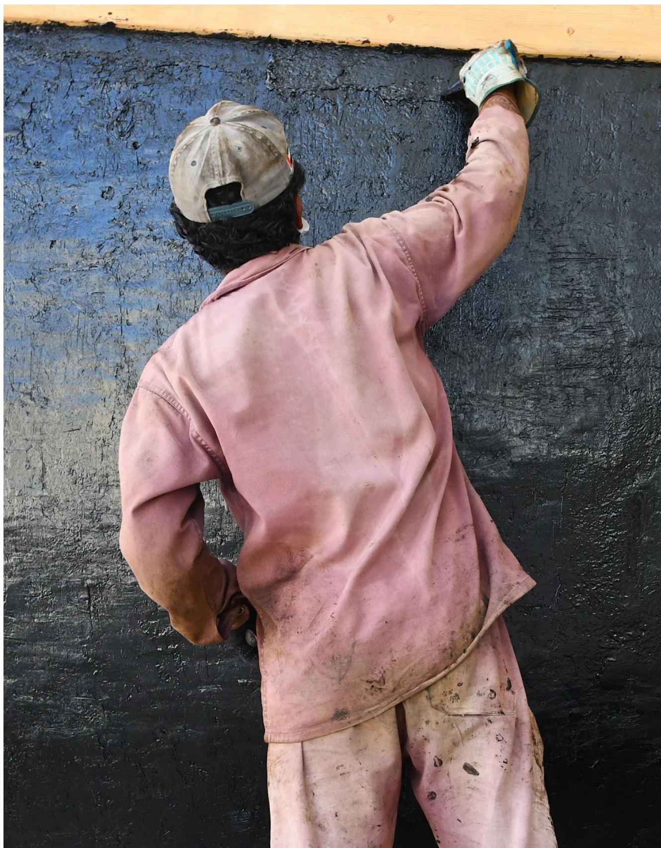
A team member helps to coat the boat with animal fat for waterproofing. Emily Harris/Zayed National Museum
