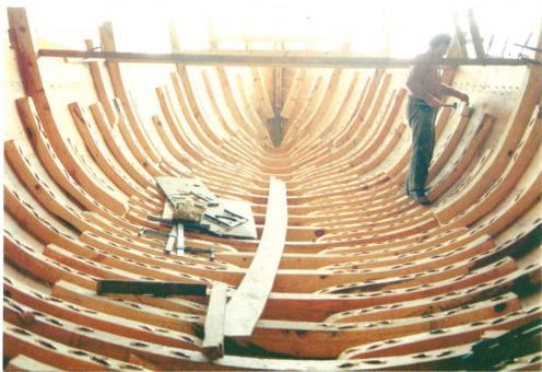
Left: Modern method of shipbuilding - the skeleton is constructed first, the shell is put up later.
