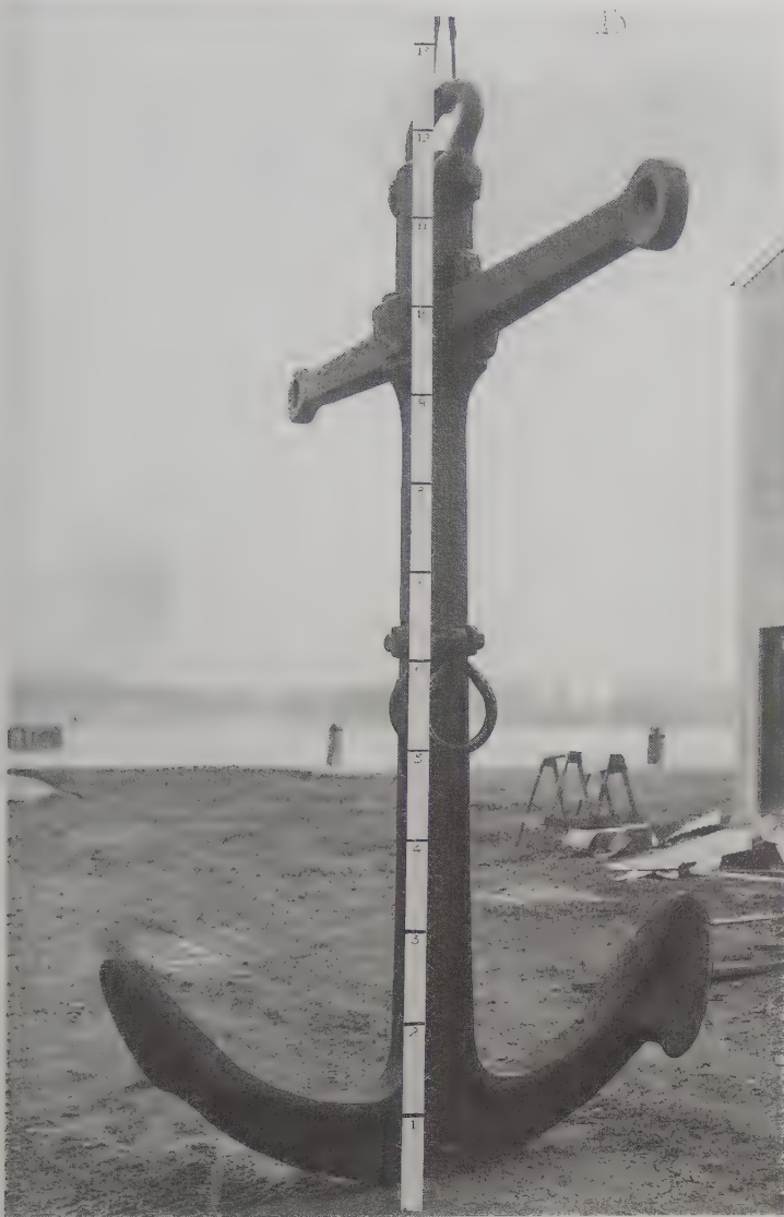
An example of Rodger's Patent Double-Concave Small-Palmed Anchor from Canada. (National Defence Photo, by RCN)
