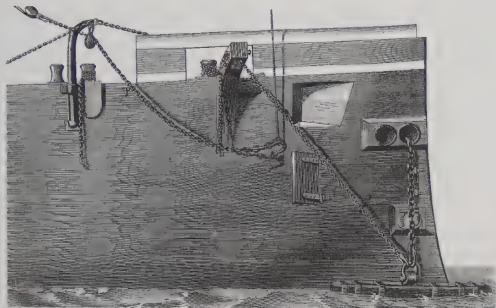
Cutting and fishing an Admiralty pattern anchor in an ironclad. (From George Nares' Seamanship, 1883 edition)
