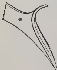
Palm detail of the Trotman Anchor. (From George Cotsell's A Treatise on Ships' Anchors , 1856)
