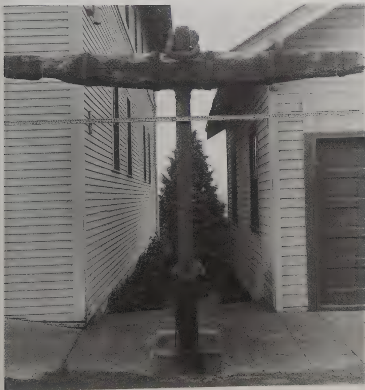
A Canadian example of a Rodger's Patent Small-Palmed Anchor. (National Defence Photo, by RCN)
