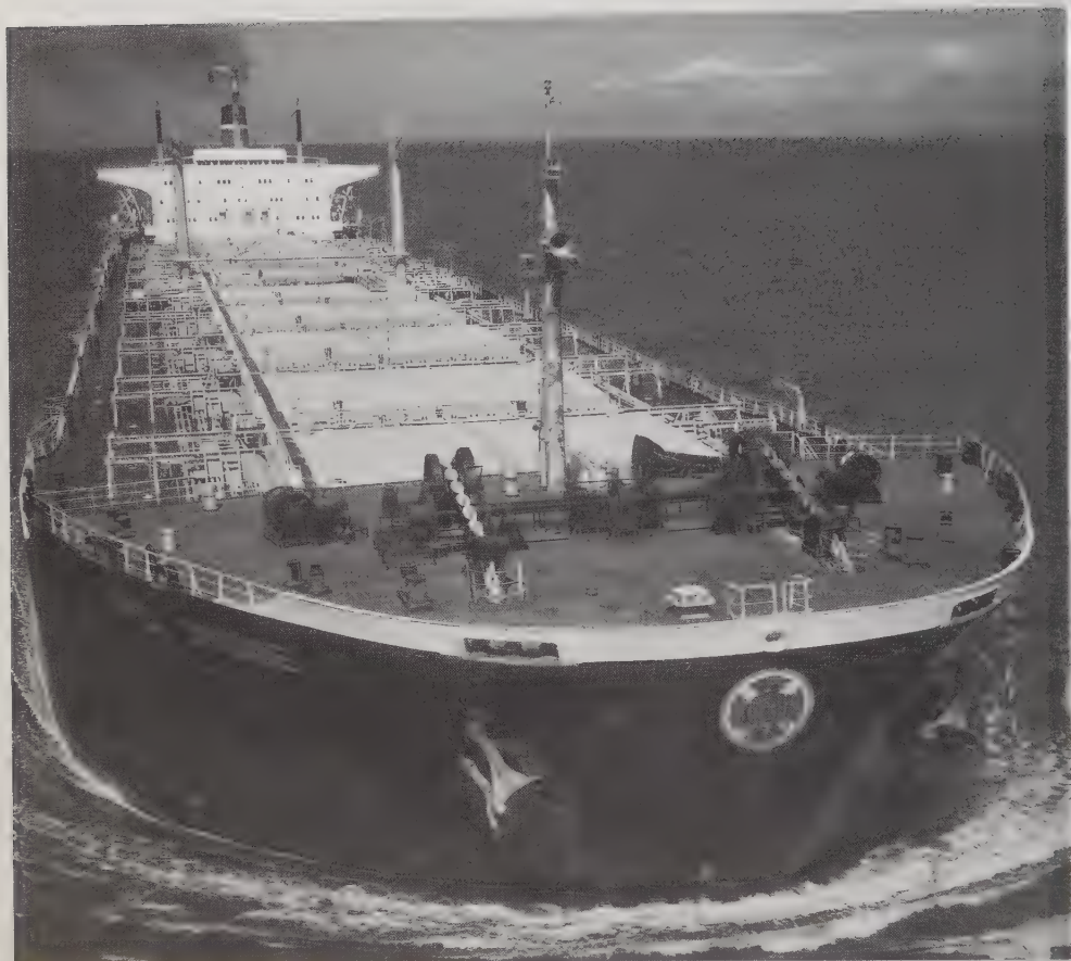
Stowage of the modern stockless anchors at the hawse pipes of the bulk carrier Spey Bridge. (Author)
