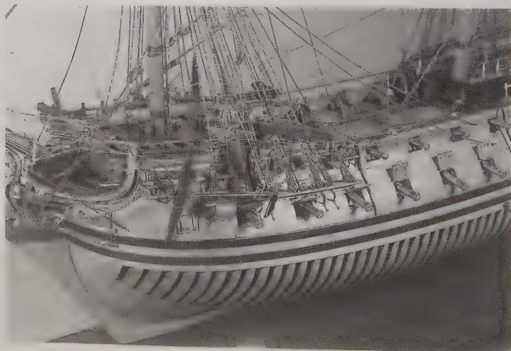
A bower anchor, its buoy, and the fish davit on a contemporary model of about 1740. (National Maritime Museum C4564a)
