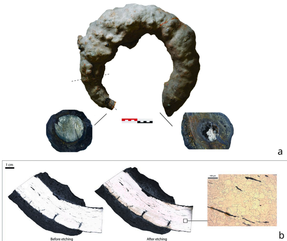
Fig. 6. a): The collected anchor ring and visualization of the state of the metal corrosion at both cut ends. b): Cross-section of the sample and metallographic observation that highlight the ferritic nature of the ring.
