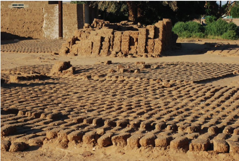
Figure 5. Modern production of sun-dried bricks in Sudan.
