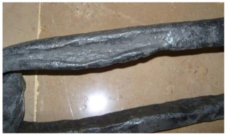
**Photograph 76:** *Physical difference in a rounded link*
