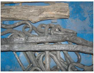
Photograph 82: Breaks in the Body of the Chain.
