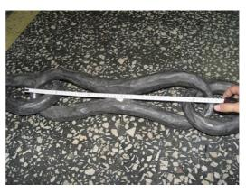
Photograph 54: Measuring the length of the link
