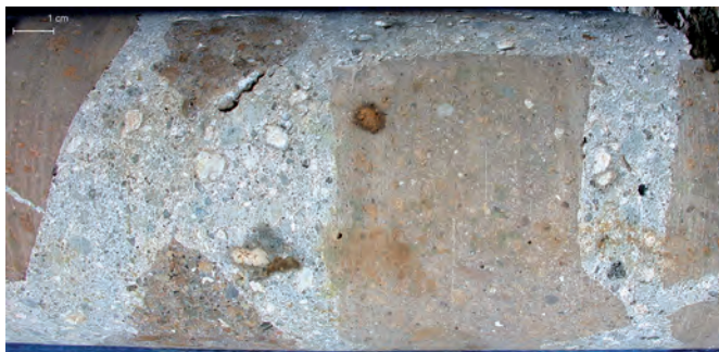
Fig. A3.26: PTR.2002.02, detail -0.60 to -0.80 m. Well-consolidated mortar with abundant sand- to gravel-sized particles of scoriaceous volcanic ash and Tufo Lionato caementa.
