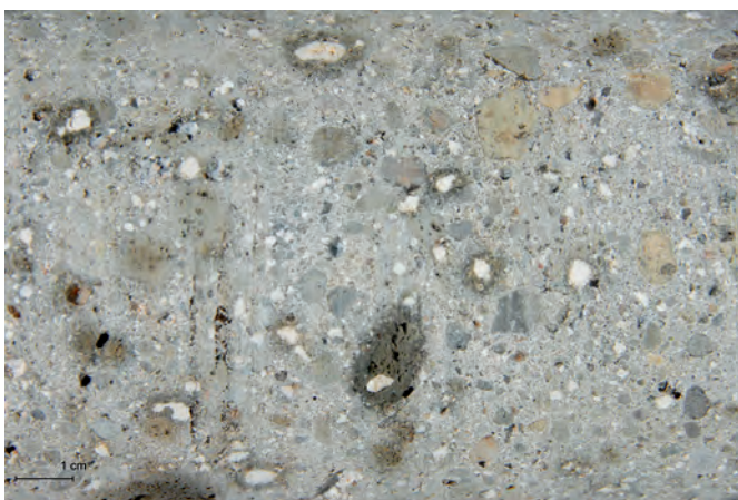
Fig. A3.36: BAI.2006.03. detail -1.90 to -1.98 m. Mortar with yellowish-gray and moderate gray pumice and glass fragments, and relict lime clasts.
