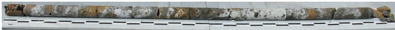
Fig. A3.34: BAI.2006.03. Overview of sea-water saturated core, with pumiceous tuff caementa and mortar with relict lime clasts. Scale bar is 10 cm.
