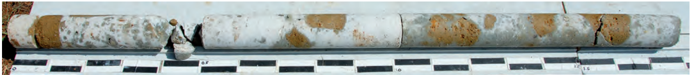
Fig. A3.48: BRI.2008.01. Overview, experimental concrete reproduction after forty-eight months hydration in sea-water. Scale bar is 10 cm.
