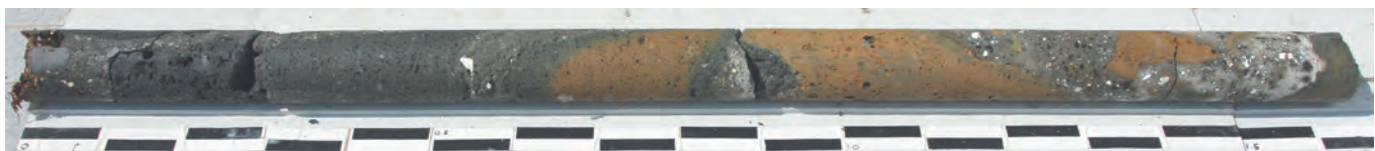
Fig. A3.38: BAI.2006.04. Overview of sea-water saturated core with abundant weathered pumiceous tuff caementa .
