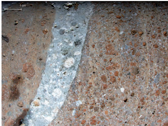
Fig. A3.22: POR.2002.02, detail -2.42 to -2.48 m. Tufo Lionato caementa with palagonitic glass and natural zeolite cements, and mortar with abundant relict lime.
