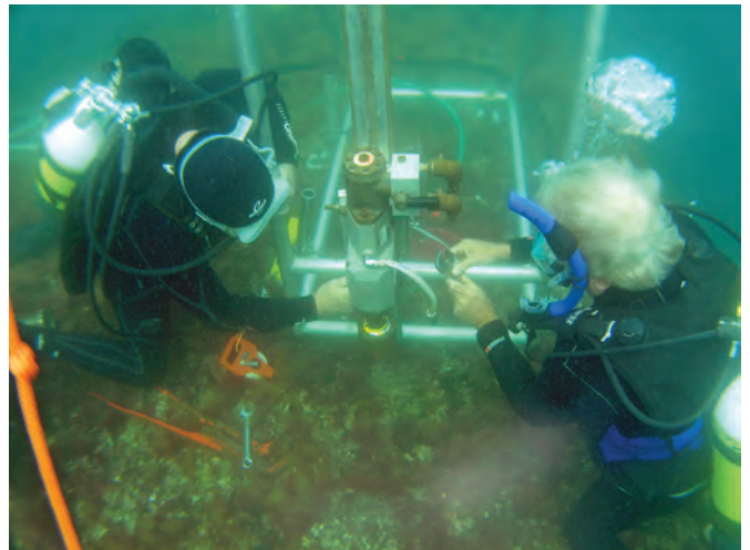
Fig. 3.41. Cordiam Hydro 25 rotary drill mounted on the M60 rack.
