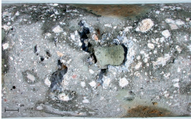
Fig. A3.16: PCO.2003.04, detail -0.20 to -0.35 m. Mortar with complex relict lime fabrics and precipitation of carbonate textures on the surfaces of compaction flaws.
