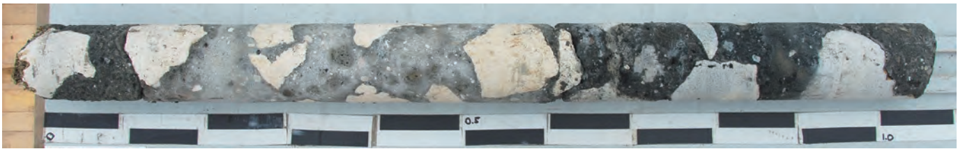
Fig. A3.71: ALE.2007.02. Oolitic limestone caementa and compact mortar with greenish-gray pumiceous ash pozzolan and relatively few relict lime clasts.
