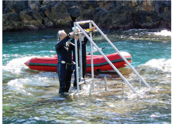
Fig. 3.40. Cordiam M60 rack being clamped to the frame at Santa Liberata.
