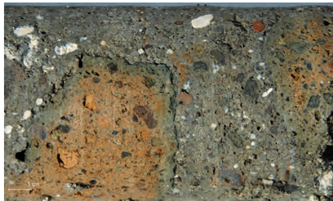
Fig. A3.40: BAI.2006.05, detail -0.40 to -0.50 m. Sea-water saturated mortar and pumiceous tuff caementa with blue-green alteration in interfacial zones.
