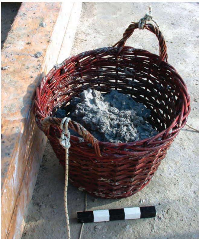
Fig. 5.14. Reproduction basket with load of mortar and ropes for lowering and dumping.
