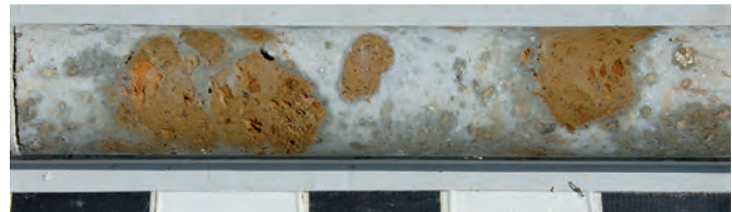
Fig. A3.49: BRI.2008.01, detail -0.65 to -0.83 m. Pumiceous Bacoli tuff and experimental mortar reproduction after forty-eight months hydration in sea-water.
