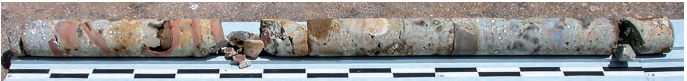
Fig. A3.10: PCO.2003.02. Overview of core, with diverse caementa , ceramics, lava, and pumiceous tuff, and a relatively low proportion of mortar, with complex relict lime clasts. The red tint is caused by rust in the core tube.
