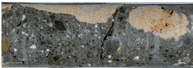
Fig. A3.42: EGN.2008.01, -1.91 to -2.18 m. Sea-water saturated calcareous sandstone caementa and pumiceous mortar with relict lime clasts.
