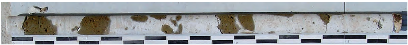
Fig. A3.43: BRI.2005.01. Overview of core, experimental concrete reproduction after six months hydration in sea-water. Scale bar is 10 cm.
