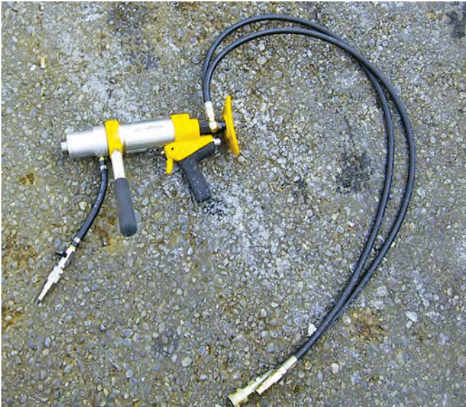
Fig. 3.22. MAG 15 hydraulic rotary hand drill.
