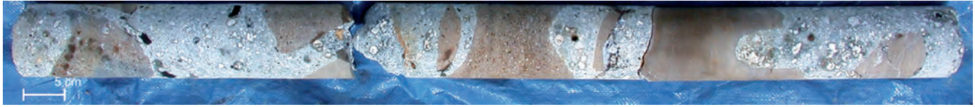
Fig. A3.20: POR.2002.02, lower sections, -1.58 to -1.98 m, and ca. -2.32 to 3.14 m. Tufo Lionato caementa, and mortar with relict lime clasts.
