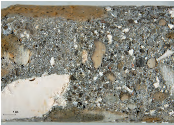
Fig. A3.32: BAI.2006.01, detail -1.60 to -1.75 m. Mortar with pale yellowish-gray glass and pumice clasts, and a large clot of relict lime.
