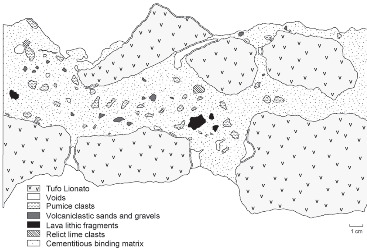
Fig. 7.5. Macroscale map of a segment of the Portus Traiani concrete, showing the principal components of the ancient Roman maritime concrete fabric.
