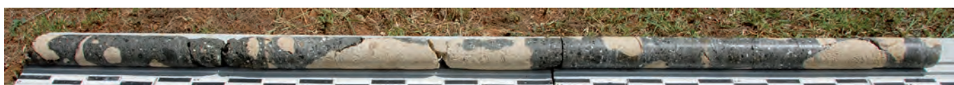
Fig. A3.41: EGN.2008.01. Overview of sea-water saturated core, with calcareous sandstone caementa . Scale bar is 10 cm.
