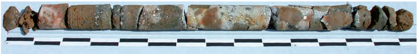
Fig. A3.1: SLI.2003.01, Overview of core. Pumiceous mortar with abundant relict lime clasts and sea-water saturated pumiceous tuff caementa. Scale bar is 10 cm.
