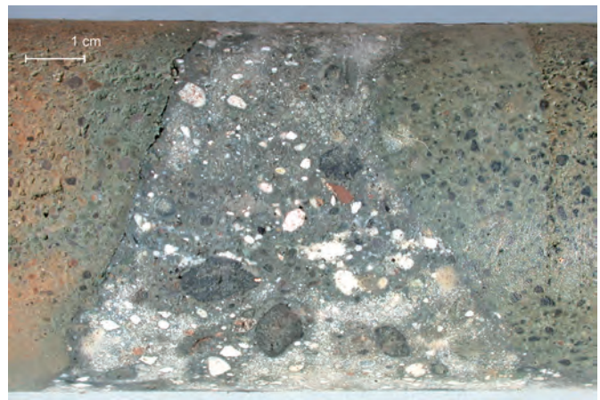
Fig. A3.6: SLI.2004.01, detail, -0.35 to -0.55 m. Mortar with abundant relict lime, particles of gravel-sized sea-water saturated volcanic glass and pumice clasts, and one ceramic fragment. The caementa are sea-water saturated pumiceous tuff on the right, and ceramic on the left.
