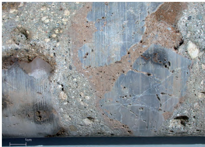
Fig. A3.12: PCO.2003.02, detail -1.25 to -1.35 m. Concrete with brown pyroclastic rock caementa , with carbonate rock lithic fragments. The origin of these rocks is not known.
