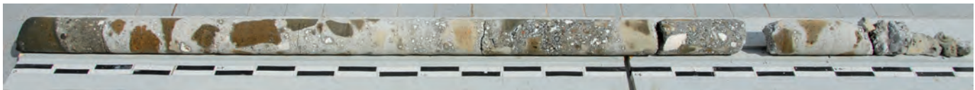
Fig. A3.31: BAI.2006.01. Overview of core, with pumiceous tuff caementa and mortar with relict lime clasts. Scale bar is 10 cm.
