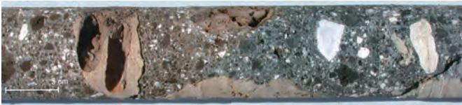
Fig. A3.67: CAE.2005.05, detail -1.30 to -1.75 m. Contact between two mortar formulations in sea-water saturated core, one with yellowish-brown pumiceous ash pozzolan (left), and one with greenish-gray pumiceous ash pozzolan (right), which also has large particles of poorly calcined limestone and calcarenite particles.
