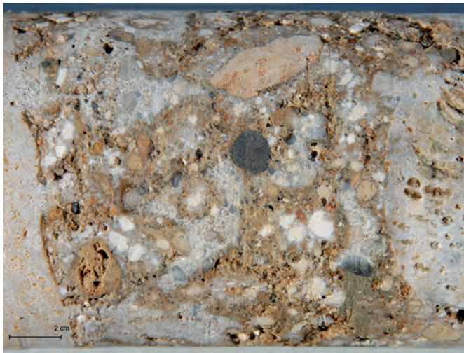
Fig. A3.55: POM.2009.01, detail -1.55 to -1.65 m. Porous mortar with pale orangish-gray pumiceous ash pozzolan and relict lime clasts.
