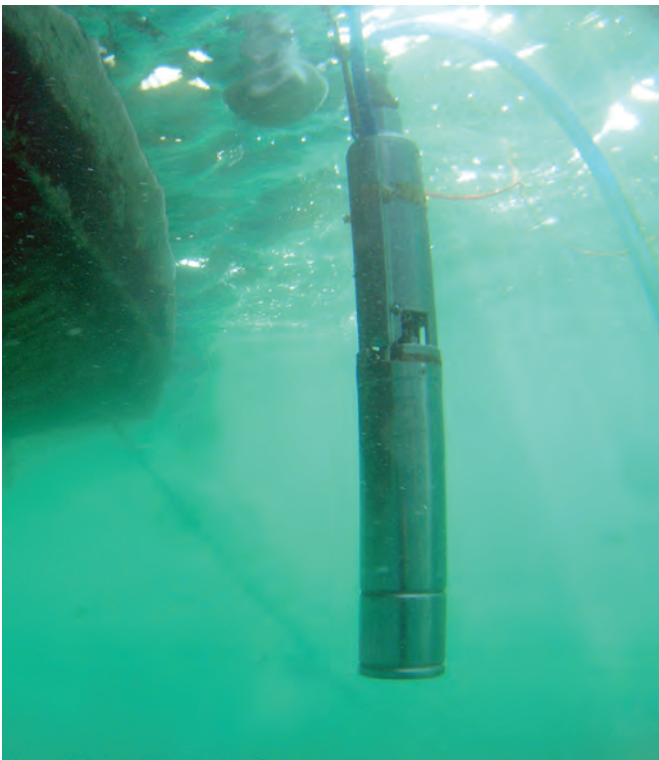
Fig. 3.23. Submersible water pump hanging off tender boat.
