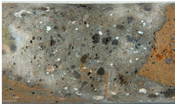
Fig. A3.39: BAI.2006.04, detail -1.20 to -1.35 m. Sea-water saturated mortar and pumiceous tuff caementa.
