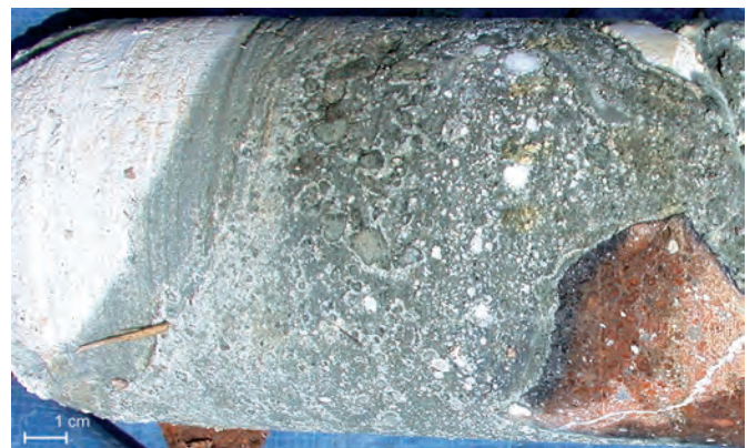
Fig. A3.27: PTR.2002.02, detail -1.35 to -1.50 m. A layer of white to light greenish-grey lime (to left) overlies light greenish grey volcanic pozzolan, and Tufo Lionato caementa on right.
