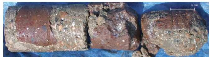
Fig. A3.23: POR.2002.03. Surviving fragment of sea-water saturated concrete with pumiceous mortar and Tufo Lionato caementa.
