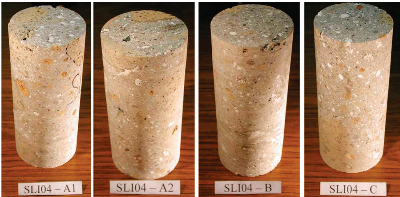
Fig. 3.10. Nine centimetre diameter core samples prepared for testing (Photo: Italcementi).
