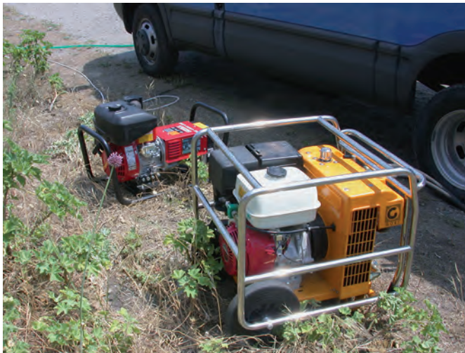
Fig. 3.20. Hydraulic fluid pump (foreground), electric generator (background).
