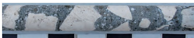
Fig. A3.76: ALE.2007.03, detail -2.15 to -2.70 m. Sea-water saturated oolitic limestone caementa and mortar with greenish-gray pumiceous ash pozzolan and relatively few relict lime clasts.
