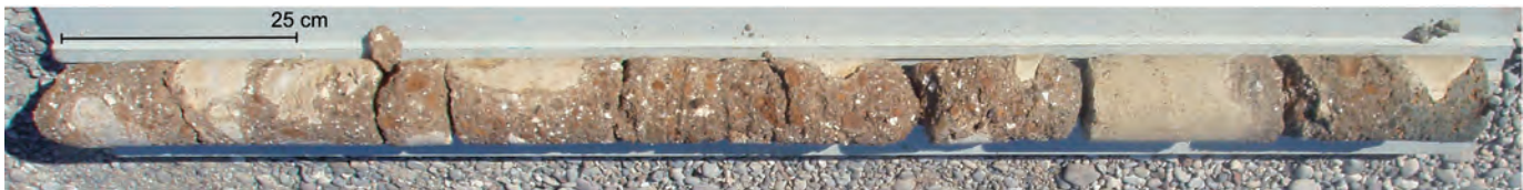
Fig. A3.51: CHR.2007.02. Overview of core, limestone caementa and porous, earthy mortar with abundant pale orange pumiceous ash and tuff pozzolan. -0.40 to -0.65 m. Scale bar is 10 cm.
