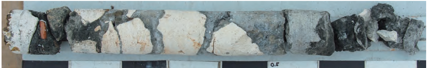
Fig. A3.69: ALE.2007.01. Overview of broken core, with oolitic limestone caementa and greenish-gray compact mortar. Scale bar is 10 cm.
