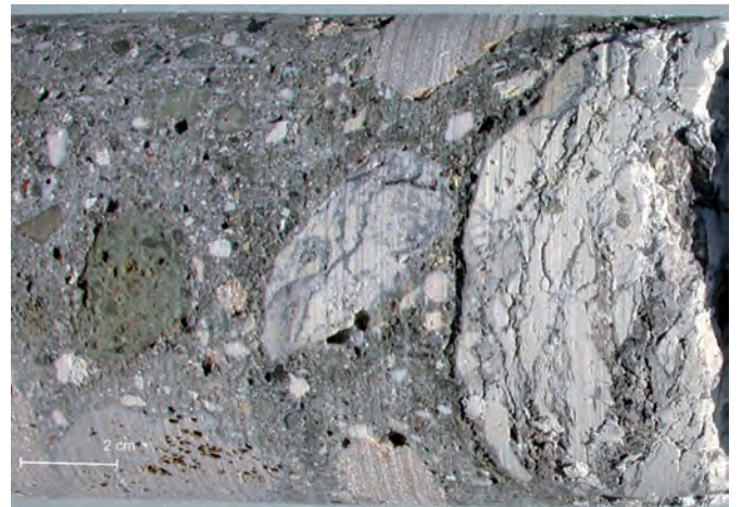
Fig. A3.61: CAE.2005.02, detail -0.28 to -0.80 m. Calcareous sandstone caementa and mortar with greenish-gray pumiceous pozzolan and relict lime clasts.
