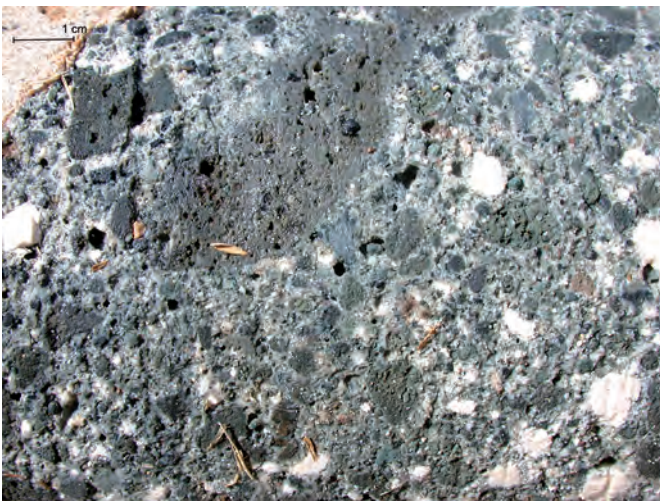
Fig. A3.68: CAE.2005.05, detail -1.75 to 1.80 m. Sea-water saturated mortar with greenish gray pumiceous ash.
