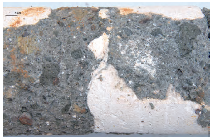
Fig. A3.78: ALE.2007.04, detail -0.55 to -0.68 m. Sea-water saturated oolitic limestone and a large clot of lime putty in mortar with abundant gravel-sized pale orange and greenish-gray pumiceous ash pozzolan.
