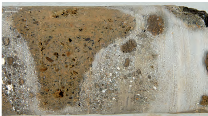
Fig. A3.33: BAI.2006.01, detail -1.85 to -2.0 m. Stratified mortar with fine ash pozzolan and relict lime at base (right), and overlain by mortar with coarse yellowish-gray pumice clasts.
