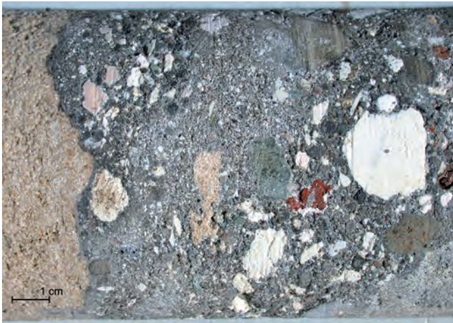
Fig. A3.59: CAE.2005.01, detail -0.65 to -0.78 m. Mortar with diverse aggregate particles including yellowish-gray pumiceous ash, clots of relict lime putty, calcarenite rock fragments, and ceramic fragments. Calcareous sandstone (calcarenite) on left.
