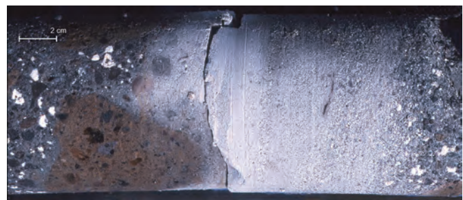
Fig. A3.30: ANZ.2002.01, detail -1.76 to -2.01 m. Stratified deposit of fine relict light greyish white lime and fine pumiceous ash.
