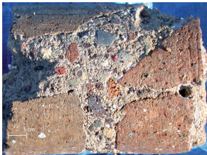
Fig. A3.19: POR.2002.01, surviving fragment, ca. -1.0 m. Concrete with Tufo Lionato caementa from the Alban Hills volcanic district, and porous mortar with scoriaceous ash likely from the Alban Hills volcanic district, yellow-gray pumiceous ash from the Campi Flegrei volcanic district (Figs. 7.10–12), and ceramic fragments.
