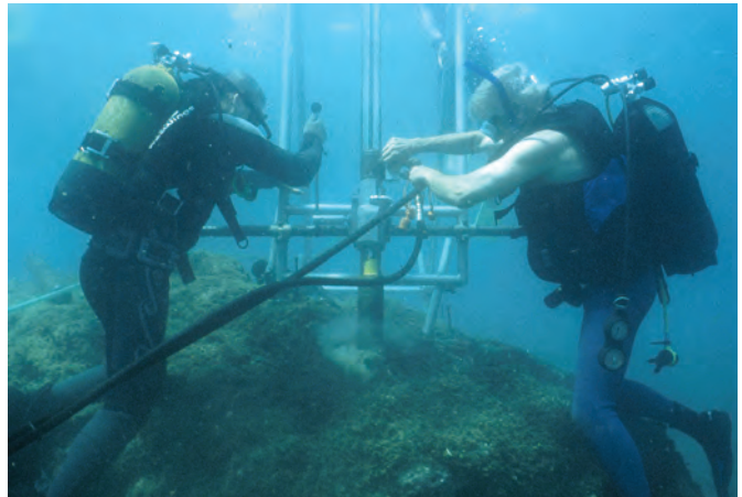
Fig. 4.16. Portus Cosanus, taking core PCO.2003.05 from Pier 5.
