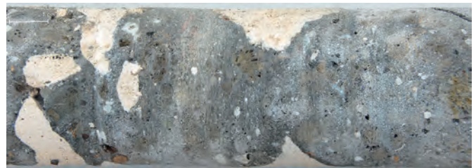
Fig. A3.70: ALE.2007.01, detail -0.15 to -0.40 m. Oolitic limestone caementa and compact mortar with greenish-gray pumiceous ash and relatively few relict lime clasts.
