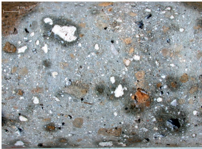
Fig. A3.14: PCO.2003.03, detail -0.98 to -1.10 m. Mortar with pale orange-gray pumice and relict lime clasts.
