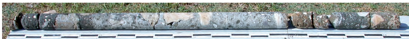
Fig. A3.64: CAE.2005.04. Overview of core, calcareous sandstone caementa , occasional pumiceous tuff caementa , and mortar with relict lime clasts. Scale bar is 10 cm.
