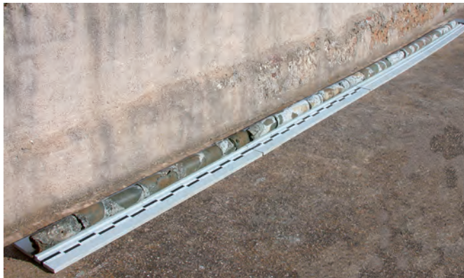
Fig. A3.3: SLI.2004.01. Overview of core, the longest recovered by ROMACONS, 5.8 m. Scale bar is 10 cm.
