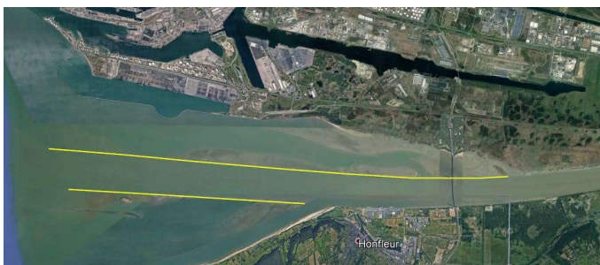
Fig. 44. River Seine estuary with north and south submersible training walls (Google Earth, 2018)
