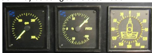
Figure 15: Triple instrument (rpm, pitch, angle)
