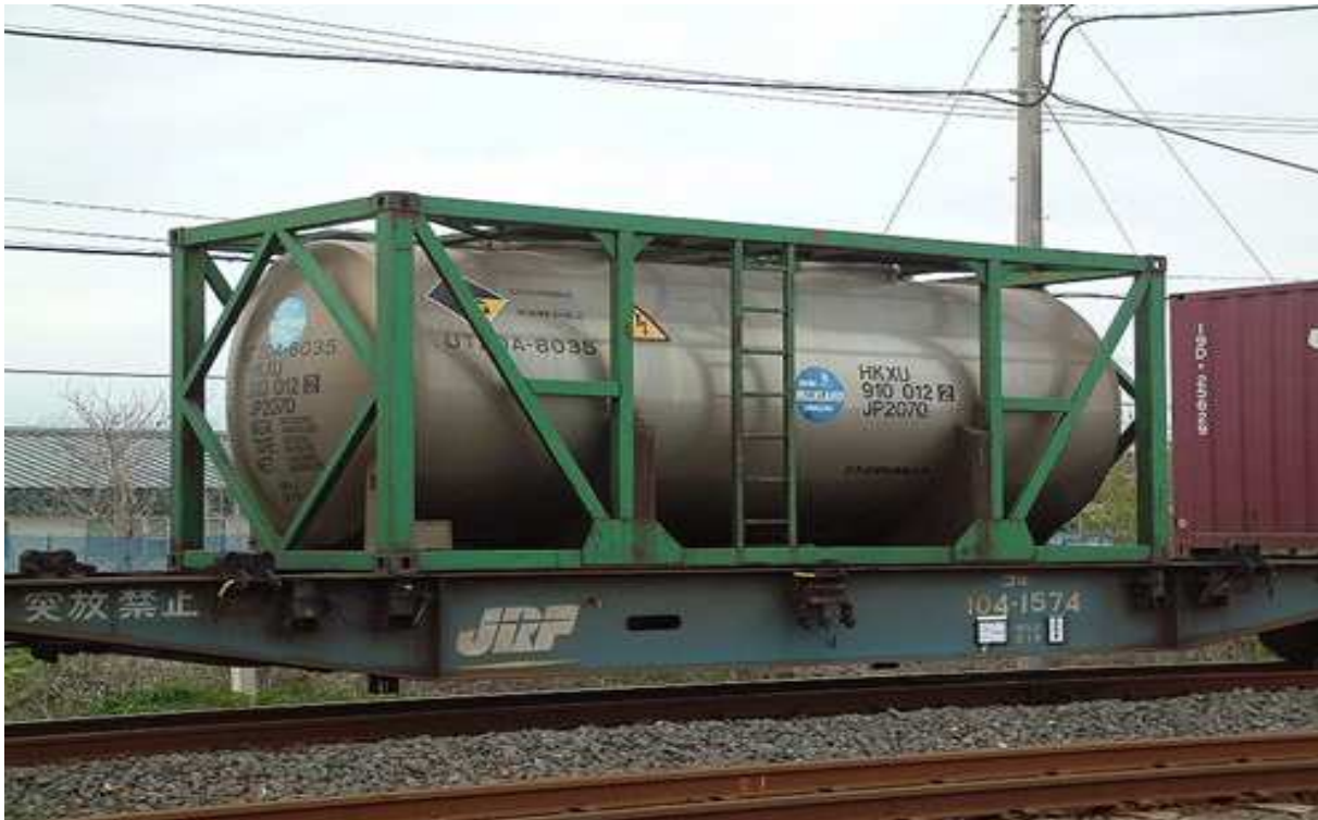
Figure 3: A standard freight tank container, (Chatama [GFDL ( http://www.gnu.org/copyleft/fdl.html ) oder CC BY-SA 3.0 ( https://creativecommons.org/licenses/by-sa/3.0/ )], via Wikimedia Commons).
