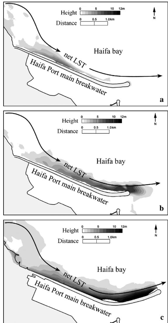
Fig. 8. Developed of the sandbar up-drift Haifa Port breakwater, see Fig. 2 for location: (a) 10 years after construction (1929–1938). (b) 30 years after construction (1929–1959). (c) 70 years after construction (1929–1998).
