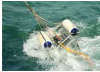
Figure 32. Shallow seismic device 'Boomer' floating on surface towed next to the fishing boat while searching for finds.
