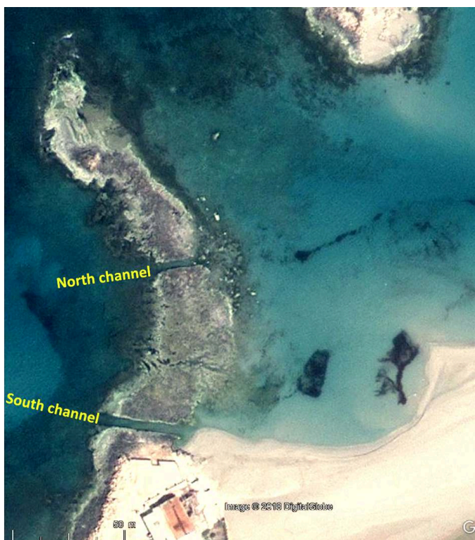
Fig. 38. El-Hanieh (Libya) western promontory with two flushing channels
