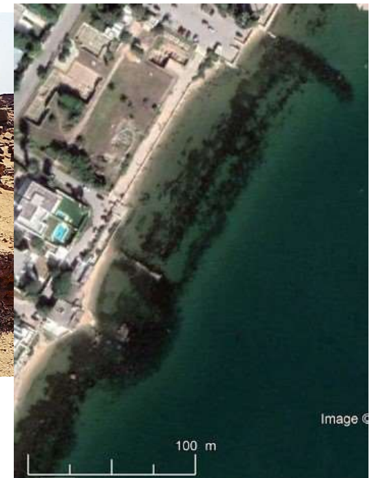
Double-line rubble-mound breakwaters at Carthage, also at Paphos, Caesarea Maritima
